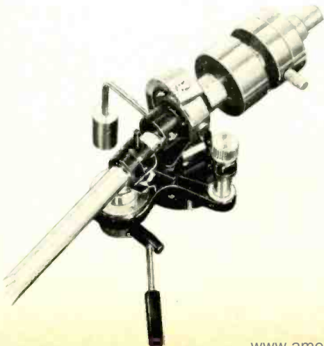
Fig. 1. Knurled knob near pickup arm's pivot adjusts antiskate force. Counterweight at left is for lateral balance. Photo courtesy Sony Corp. of America.
