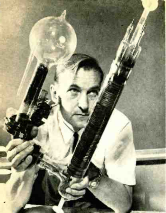
RCA sun bottle: First gas lasers to produce intense rays of ultraviolet light continuously up to 1000 hours, to be used to solve mysteries of life.
